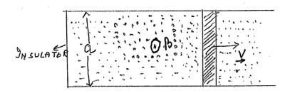
9-6. Same situation as in problem 9-5 but now there is a resistor  $R = 2\Omega$  between the rails. (i) What is the current in the circuit? (ii) Now do you need a force to move the rod?
